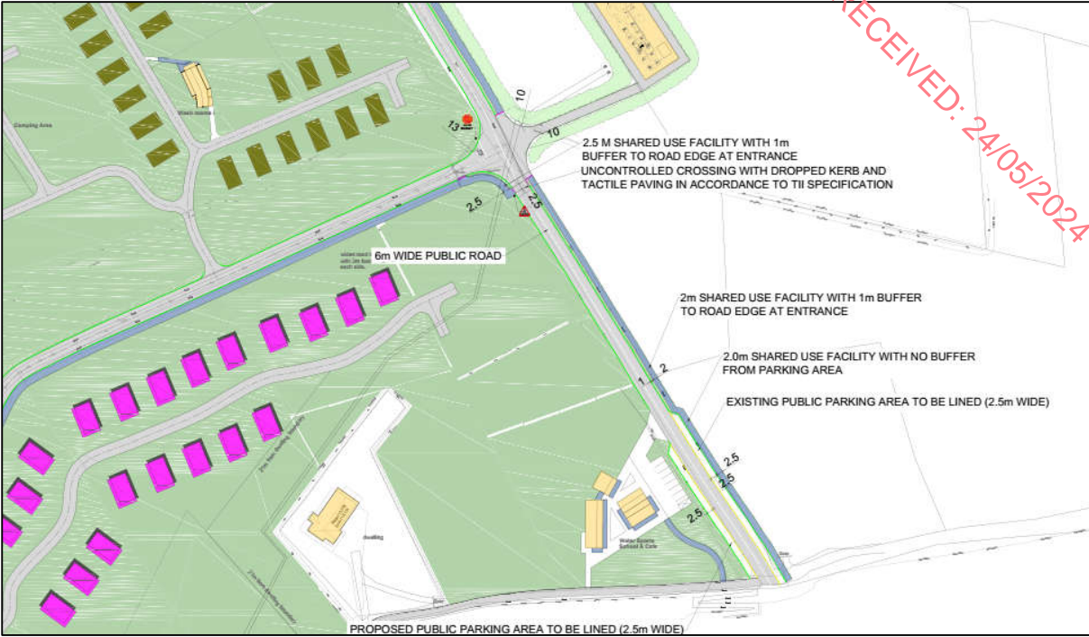
Figure 2-18: Section of the road network including the upgrades to the beach access road (L-7535), the WWTP entrance and the main entrance to the Hotel and Leisure Park with details of road and path widths.
